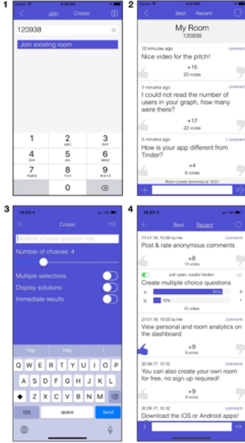
Fig. 1. Screenshots of the SpeakUp mobile app. (1) Joining a chatroom. (2) Viewing messages in the chatroom ordered by time or score. (3) Creating a multiple choice question in the chatroom. (4) Visualizing the results of a multiple choice question.
